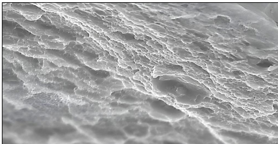
Figure 3. 13 SEM Micrograph (Meg = 5KX) of Al-Alloy (6061) of Aging for 8 Hours
